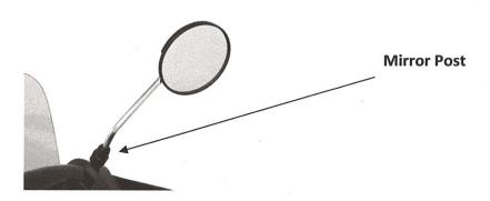
To attach the mirrors simply place each mirror threaded end into the mirror post. Turn mirror clockwise and fasten mirror to scooter.
