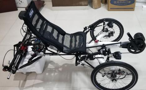
2. Remove the bolt on rear right axle with a 8mm Allen wrench.
