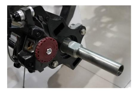
3. Remove the bottom bolt of rear caliper with a 4mm Allen wrench. Put up the caliper and get the right wheel through right axle.
