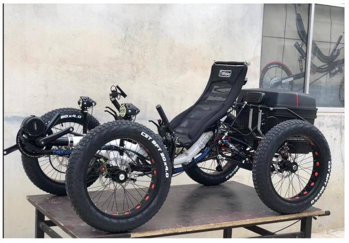
Your quad is properly tuned by our engineers before it was shipped out. The rear brake rotors may be not in the center of the calipers when you fit the two rear wheels. You need to check the screws on the calipers.
