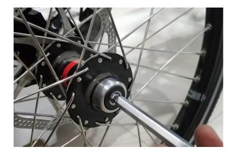
4. Finish the assembly of right wheel. And fit the left wheel by the same way.
