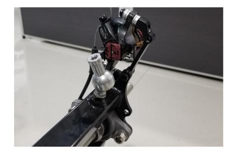
Put down the caliper and tighten the bolt.
