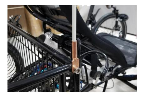
8. Fit the pedals and put the front boom straight, adjust it according to your x-seam and tighten the bolts on caliper ring with a 6mm Allen wrench.
